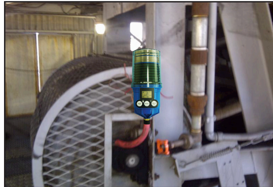
Automatic lubrication systems now provide just the right amount of grease.
